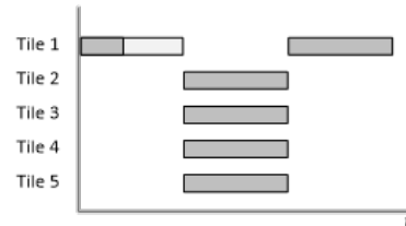
Fig. 3. Example for task dependencies in a multicore architecture
