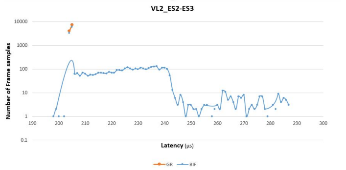
Fig. 7: Virtual Link 2 (End system 2 to End system 3) observation for Jitter.
